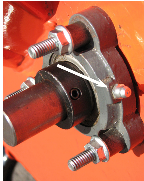
Figure 5.13, Chute Side Bearing Zerk
