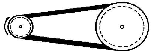
ENGINE DRIVE PULLEY 10,000 \text{ RPM} \pm 500 \text{ RPM} = 4750\text{-}5250 \text{ RPM} WHEEL SPEED
